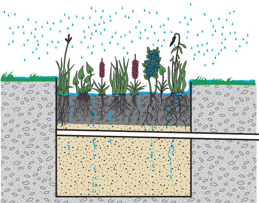
**Biofiltration devices are designed with special soils, storage areas and drains.**
